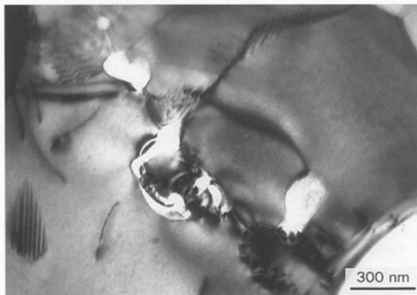
Figure 3 Defects in the alumina matrix of the composites (TEM).
